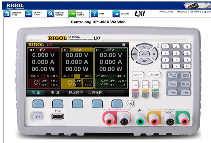
Figure 3-5 Control DP1308A via web
